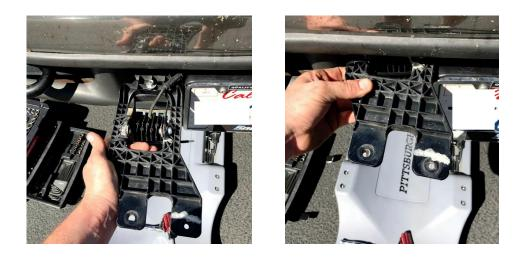
11. Attach the plug 'n play adapter to the factory harness and the Squadron power cord. Repeat this step for the other side. Tie the wires away from any hot and/or rotating components.
